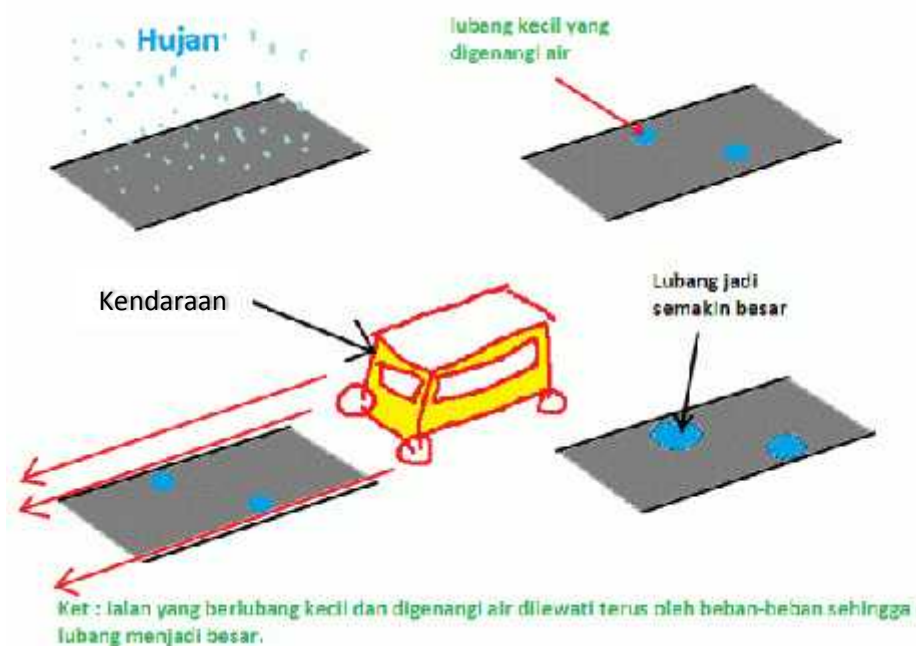
Gambar 6.1 Proses jalanan berlubang
