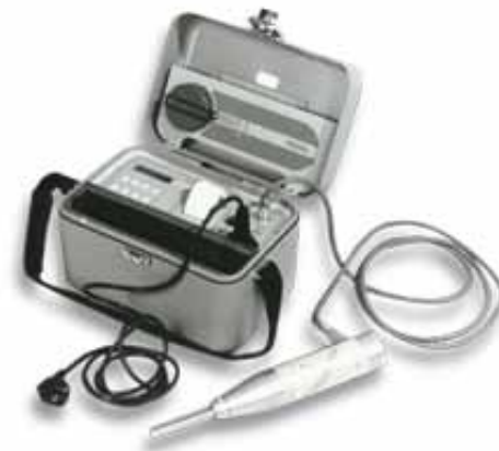
Gambar 4.1. Alat Hammer Test
