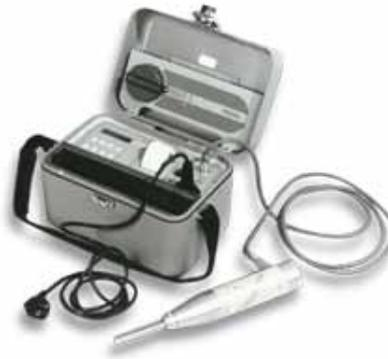
**Gambar 2.9. Hammer Test**
