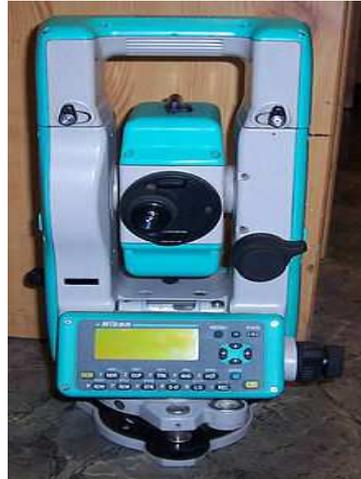
**Gambar 4.1** Contoh Teodolit Elektronik (Total Station)
