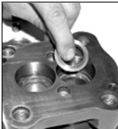
Gambar 4.38 Melepas Ring seal
