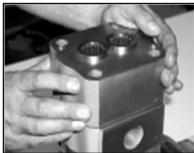
Gambar 4.91 Memasang Bearing carrier
