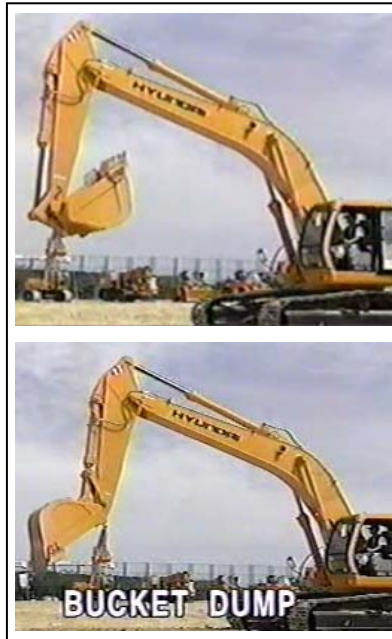
Gambar 4.19 – Pengetesan bucket dump
