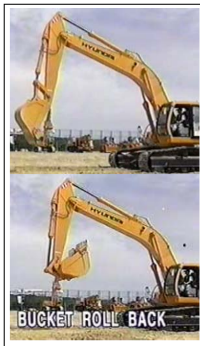
Gambar 4.18 – Pengetesan bucket roll back
