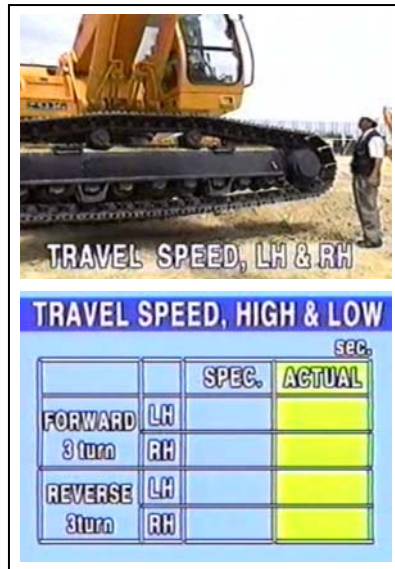
Gambar 4.21 – Pengecekan travel speed
