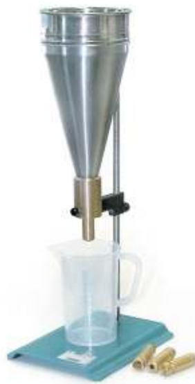
Gambar 5. 2. Grout flow cone set
