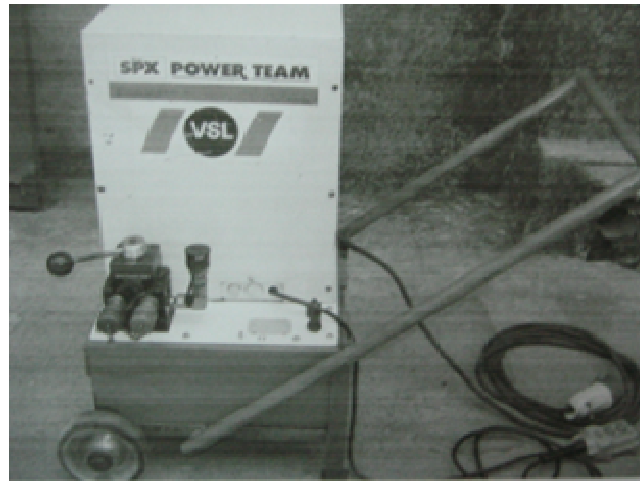
Gambar 4. 5. Hydraulic Pump PQ 1204 (3 Phase)
