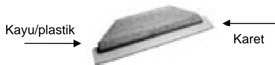
Gbr. 4.20 Karet " grouting "
