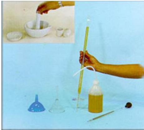
Gambar 5.e6 Funnel, Burette, Evaporating Dish, Mortar and Pestle, Wash Bottle, Pipette, Crucibles
