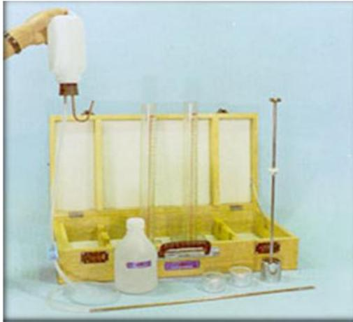
Gambar 5.b10 Sand Equivalent Test Set
