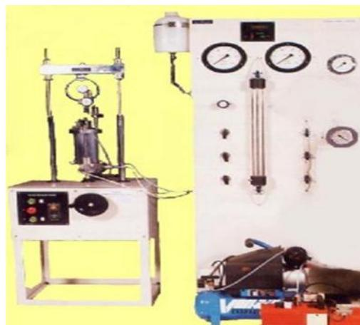
Gambar 5.a22 TRIAXIAL TEST SET, Digital reading pore pressure
