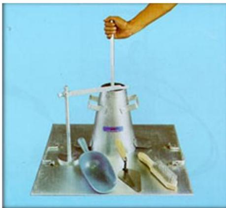
Gambar 5.c10 Slump Test Set
