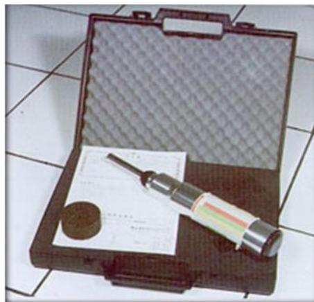
Gambar 5.c7 Concrete Test Hammer
