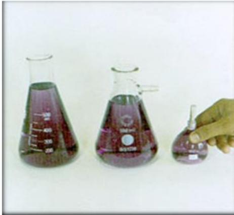
Gambar 5.e5 Erlenmeyer Flask, Vacuum Flask, Density Bottle
