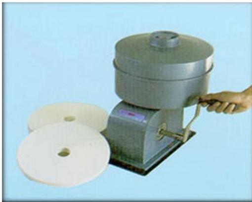
Gambar 5.g2 Centrifuge Extractor Test Set
