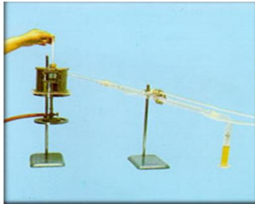
Gambar 5.g4 Distilation Of Cutback Asphalts
