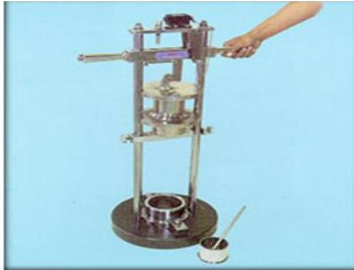
Gambar 5.b1 Aggregate Impact Test
