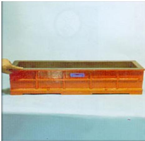
Gambar 5.c4 Concrete Beam Mold
