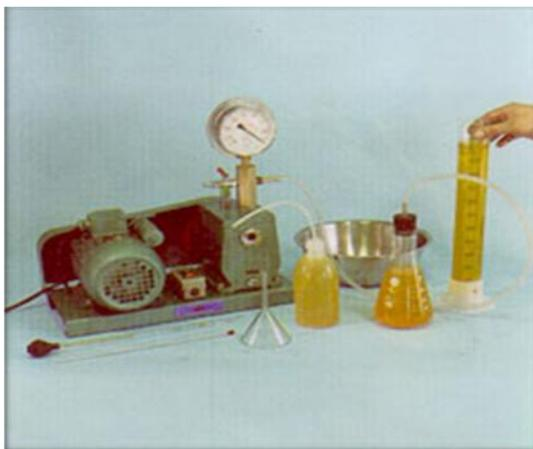
Gambar 5.a19 Specific Gravity (Vacuum Method)
