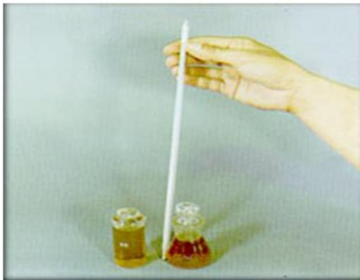
Gambar 5.g14 Specific Gravity of Semi-Solid Bituminous Materials
