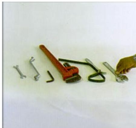
Gambar 5.e10 Open End Wrench, Ring Spanner, Allen Key, Pipe Wrench, Strap Wrench, Adjustable Wrench
