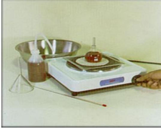
Gambar 5.a17 Specific Gravity (Heating Method)
