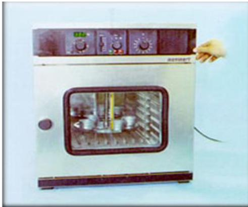
Gambar 5.g8 Loss on Heating/Thin-Film Test
