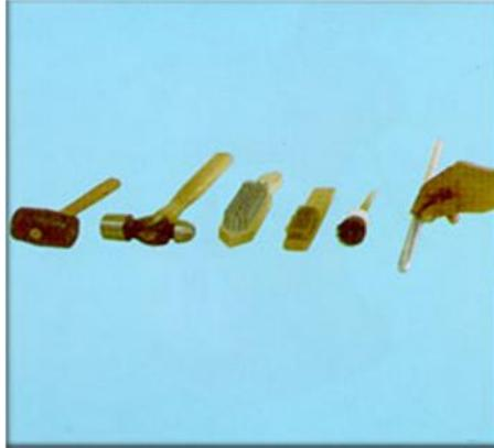
Gambar 5.e14 Rubber Mallet, Hammer, Steel Wire Brush, Brass Wire Brush, Soft Brush, Tamping Rod
