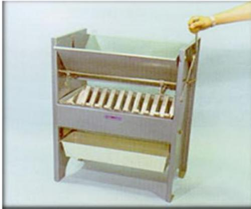
Gambar 5.b4 Gilson Sample Splitter
