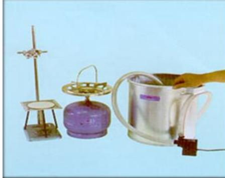
Gambar 5.e2 Cooling System, Butae Field Heater, Bunsen Burner, Statif, Tripod Stand, Asbestos Wire Gauze
