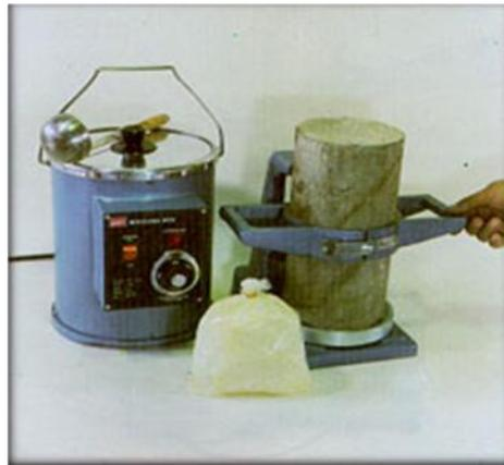
Gambar 5.c11 Vertical Cylinder Capping Set
