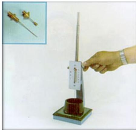
Gambar 5.d4 Time of Setting of Hydraulic Cement by Vicat Needle
