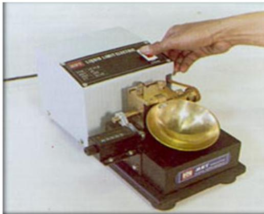
Gambar 5.a10 Liquid Limit Device
