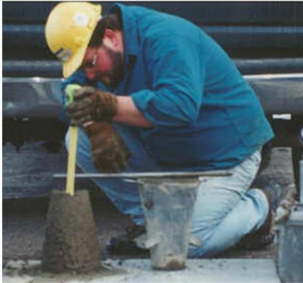
Gambar 5.4.4.Slump test
