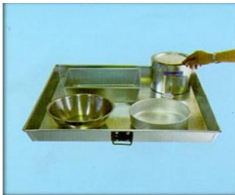
Gambar 5.e16 Square Pan, Rectangular Pan, Round Pan, Mixing Bowl, Sample Can, Thin Box
