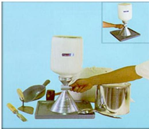
Gambar 5.a15 Sand Cone Test Set
