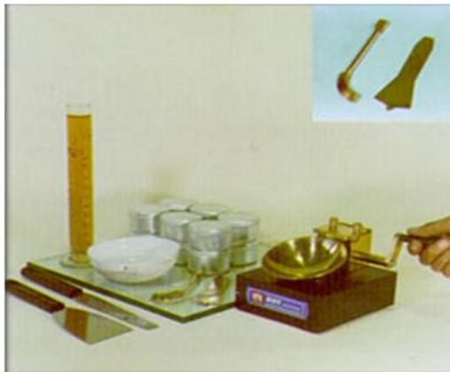
Gambar 5.a11 Liquid Limit Test Set
