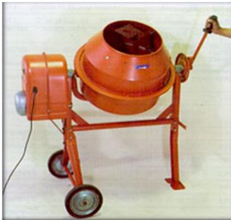
Gambar 5.c9 Laboratory Concrete Mixer
