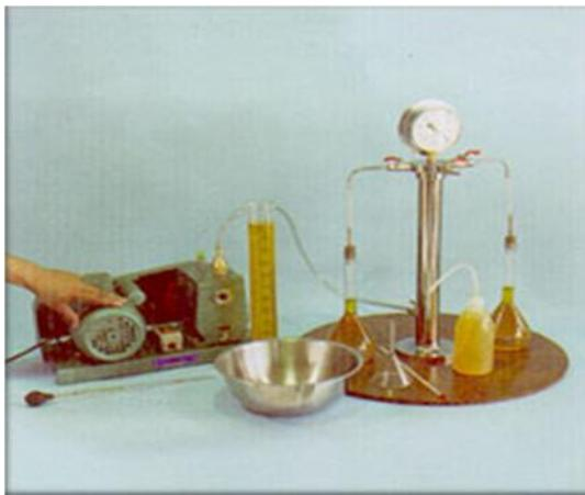
Gambar 5.a18 Specific Gravity (Vacuum Method)
