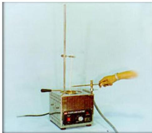
Gambar 5.g6 Flash and Fire Point by Cleveland Open Cup
