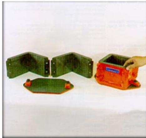
Gambar 5.c5 Concrete Cube Mold
