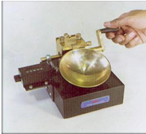
Gambar 5.a9 Liquid Limit Device
